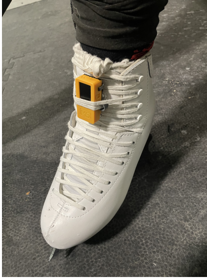
Figure 3. M5StickC Plus2 placement on Figure Skater boot
